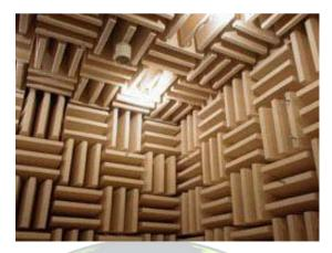
An Anechoic Chamber, Using Acoustic Absorption to Create a "Dead" Space
